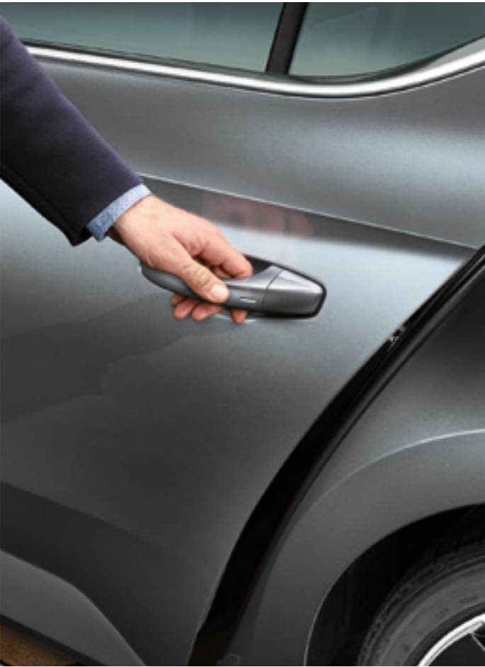
KESSY With the new version of the KESSY (Keyless Entry, Start and exit System) all doors can be used to unlock or lock the car.
