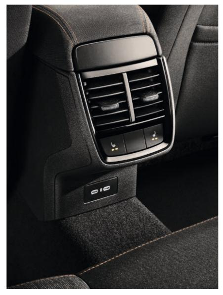
**HEATED SEATS / USB** In cold weather, your friends and family will appreciate the heated rear seats, which are regulated by a separate control on the rear side of the front armrest. Two USB-C slots enable universal mobile phone charging.
